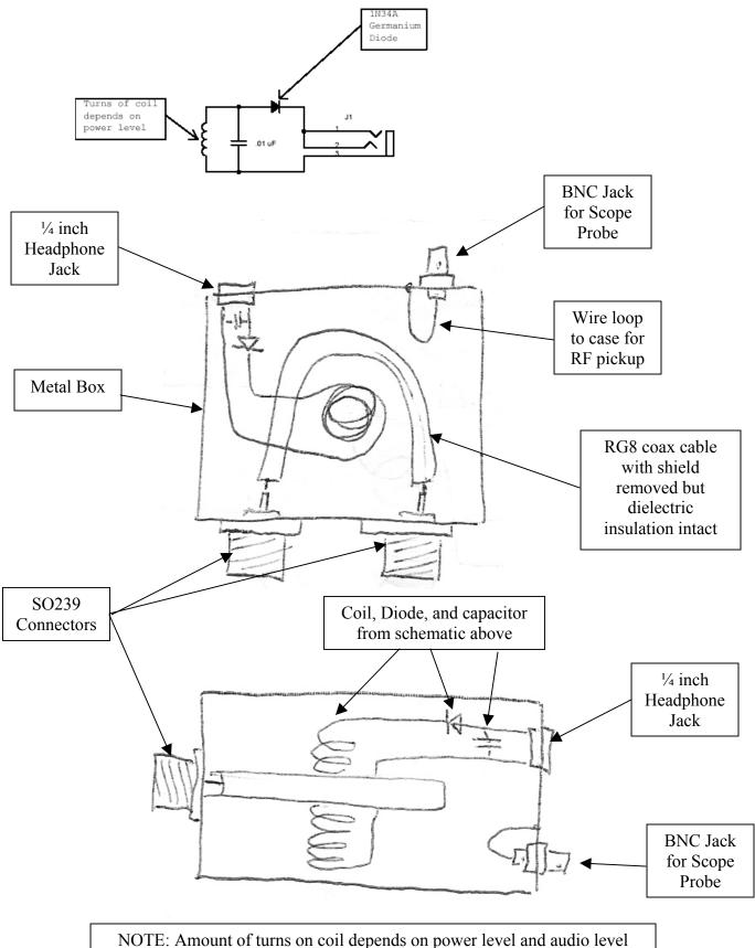
NOTE: Amount of turns on coll depends on power level and audio level desired. More turns produces louder audio for any given power level. Heavier gauge wire provides better mechanical support for the coil structure
